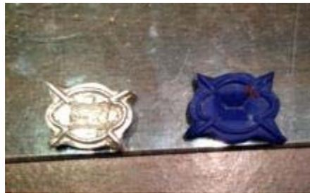
The next steps are cleaning up the casting, adding prongs to the piece to hold the stone in. add a tube to the back to hold the cord, pre polish, polish, add the center stone, and lastly attach the pearls.
