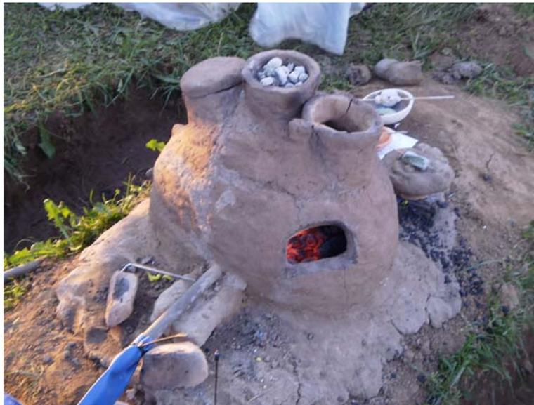
As you can see the front has an opening to reveal the hot coals, the top side openings are vents to help regulate heat, air flow and a work port. The center top opening is an annealing chamber. It worked quit well. Pictured below is the furnace in use.
