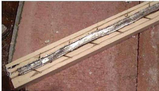
3) After I pulled the lead from the mold, I cut off all the lead from the sprues and cleaned up the edges.
