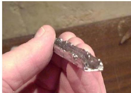
For the solder, I took one part lead to five parts tin (Theophilus pp56). I melted them together and used the lead came mold to form the solder (Photo G). As Theophilus described there is no reason to make a mold when you already have one.
