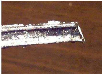
3) I used a knife to trim off the rough edges along the top of the lead. Photo I shows the same piece of lead now trimmed.
