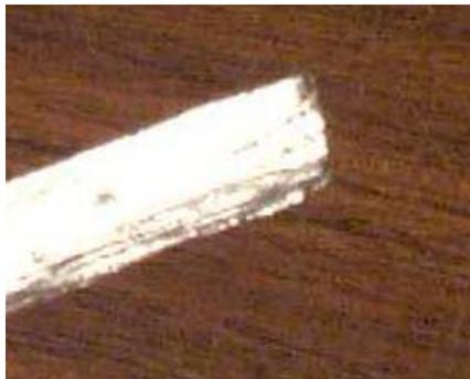
4) I made the solder by melting 1 third lead to 2 thirds tin and cast it in the same mold that I used for the lead (see appendix A – solder).
