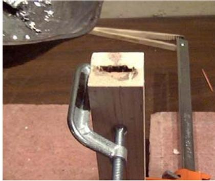
1) I used the mold as shown in Photo G to create the H shaped lead comes. To create the U shaped comes, I simply reversed one of the blocks of wood.
